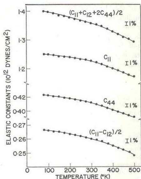
FIG. 3. The temperature dependence of elastic constants of MgCu<sub>2</sub>.
